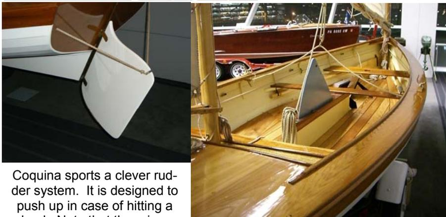
Coquina sports a clever rudder system. It is designed to push up in case of hitting a shoal. Note that there is no tiller. The rudder is easily controlled by a continuous line that goes all the way to the bow. You can steer the boat while you are at the foremast putting up the sail.
